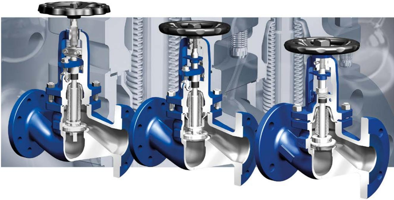
**Fig. 2:** Selection of stop valves with a bellows seal: the FABA-Supra C with two-piece stem and medium-flushed bellows (left), the FABA-Supra I with bellows cover (centre) and the FABA-Plus (right).
