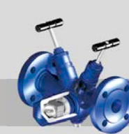
Steam traps with multi- valving technology CONA® "All-in-One" (incl. stop valve, inside strainer, back-flow pro- tection, drain valve)
