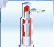
Integrated sensorics, proximity switch; used to return the feedback signal to the control room.
