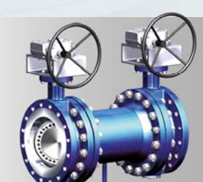
Double block & bleed (DBB) provides safe double blocking with the void monitored and optional pressure relief to atmosphere.
