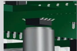
Contactless and precise stroke determination with the Hall sensor enables wear-free use even in harsh conditions
