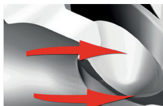
Improved control characteristic due to throttling plug with a flow friendly shape
