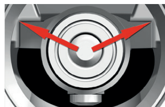
Standard non-rotation feature due to double guided plug in the body
