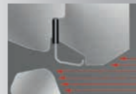
The protection of the seat sealing ring against the influence of negative medium flow creates a long service life of the ZEDOX®
