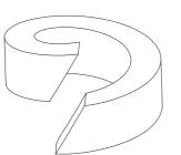
Fig. 20: Stuffing box packing
