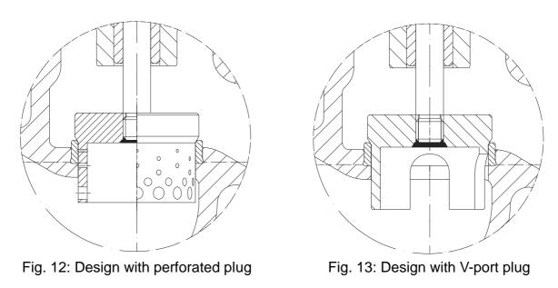
(Design with pressure balanced plug refer to Fig. 27)
