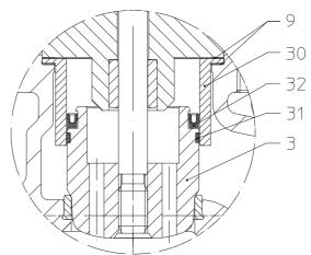
Fig. 27: Pressure balanced plug
