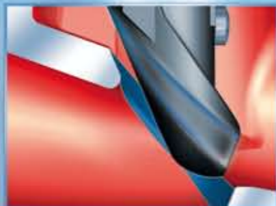
1. Increased durability due to the gentle insertion of the self aligning plug into the seating area
